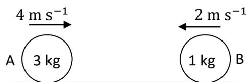
Spheres A and B are moving towards each other with speeds of  $4 \text{ m s}^{-1}$  and  $2 \text{ m s}^{-1}$ , respectively.
