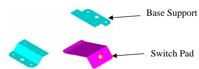
**Base supports** - The accurate positioning of the  $\text{Ø}4.5$  drilled holes was critical to the assembly of the finished artefact. Marks were gained by candidates who:
