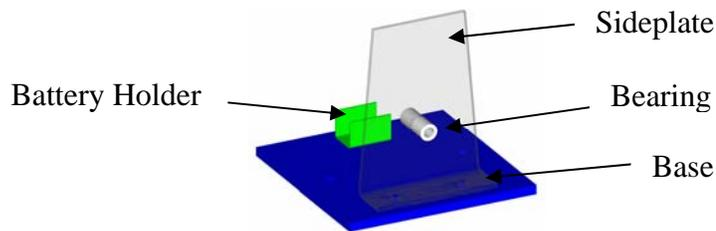
**Base** – Most candidates achieved good marks as the base generally was the correct size and was drilled and tapped correctly. Some candidates failed to engrave their examination number on the top surface of the base as per the *Instructions for making the project*.
